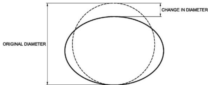
$$\% \text{ DEFLECTION} = \frac{\text{CHANGE IN DIAMETER}}{\text{ORIGINAL DIAMETER}} \times 100$$
