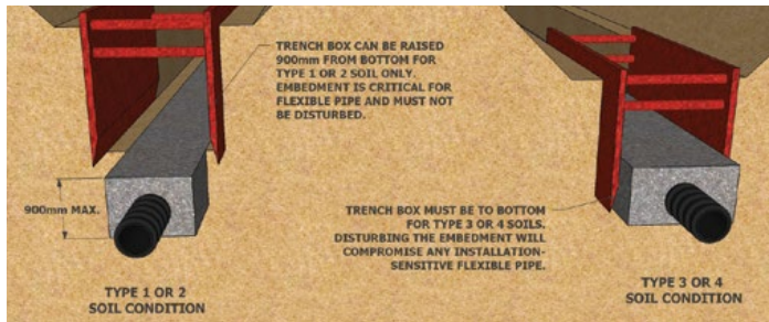
Proper use of a trench box
