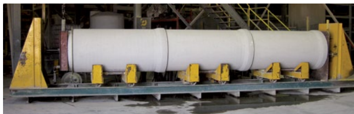
Hydrostatic test of concrete pipe
