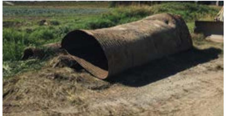
*Severely corroded corrugated steel pipe*
